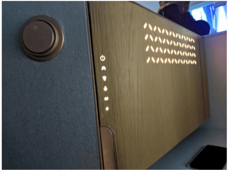
Panasonic/Colins Aerospace Element - Non intrusive light and controls on any surface
