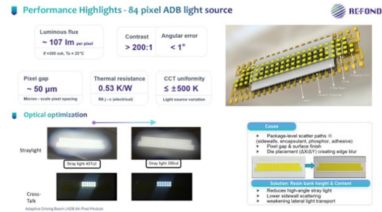
84 pixel ADB highlights and optical optimization
