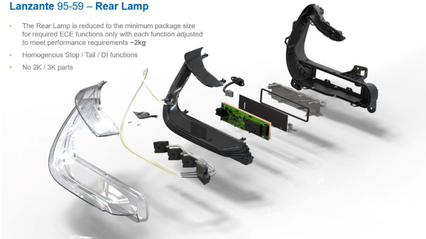
Rear lamp exploded view: integration of Luxibright optical fibers and remote light sources
