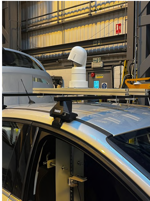
Figure 4: Camera for ANPR installed on the trials vehicle (camera shown in “power off” orientation)
