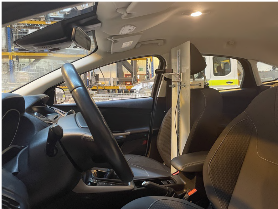
Figure 3: Luminance camera installed at RHS driver eye height. During trials the mounting plate was covered with black cloth to prevent reflection in the windscreen
