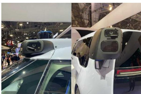
Waymo's latest robotaxi is based on a Zeekr minivan. Reducing cost of the hardware was a primary goal, so front and rear lidars have been removed; the corner lidars now cover a wider field of view, and the system has HD radar. Another improvement was to better weatherproof the sensors; there are now wiper blades on the cameras. These cars are already testing in San Francisco and other markets.
