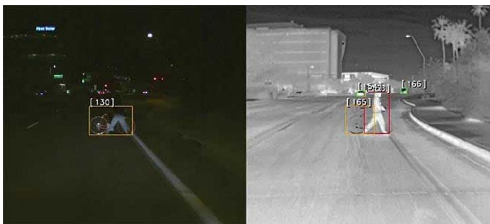
A scene as seen by a standard camera (L) and a thermal camera (R)
