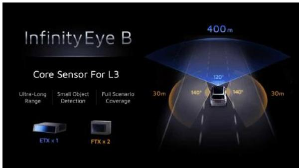
Tailored for  $L^3$  conditional autonomous driving systems, it has a forward-facing, long-range ETX lidar and two FTX lidar for blind-spot detection. This multi-lidar configuration balances extended ranging capability with wide-angle field-of-view perception, essential for  $L^3$  driving tasks, where the vehicle self-drives in certain situations while allowing for human intervention.
