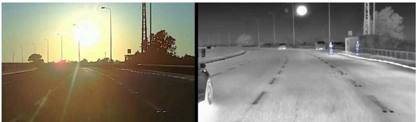
Thermal imaging cameras from Adasky can detect a pedestrian crossing a road with his bicycle at night, revealing hazards invisible to visual spectrum cameras and ensuring safer autonomous navigation in low-visibility conditions
