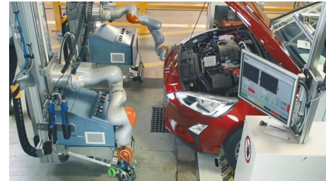
Example of Aiming Station Source: Dürr
