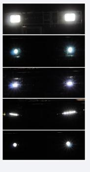
Illuminance assessed in a distance of 50 m and 37.5 m. Area: light emitting area (outer dimensions) for one headlamp, does not correlate with a homogenous luminous area
