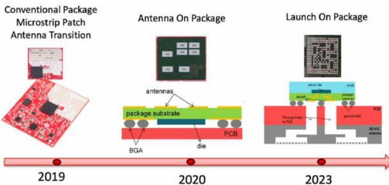
The more advanced LoP (launch on package) technology is being used by Continental in the production of their sixth-generation radar chips. LoP enables the electromagnetic waves emitted by the radar to propagate directly from the chip through the air waveguide, avoiding the higher energy loss and high cost caused by etching the antenna on the circuit board, achieving low cost and improving the radar's detection performance.
