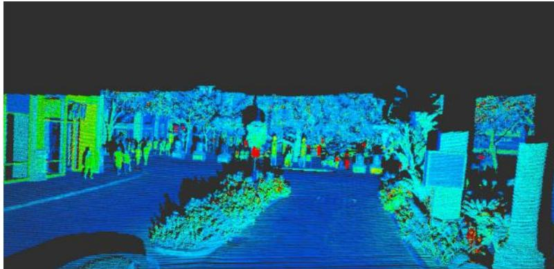
directional lidar focuses on specific, predefined areas. This targeted approach allows for higher resolution in detection, essential for identifying minor movements or small objects that rotating systems might miss. In security settings, where every detail is critical, having a sensor that provides consistent and precise data is a notable benefit.
