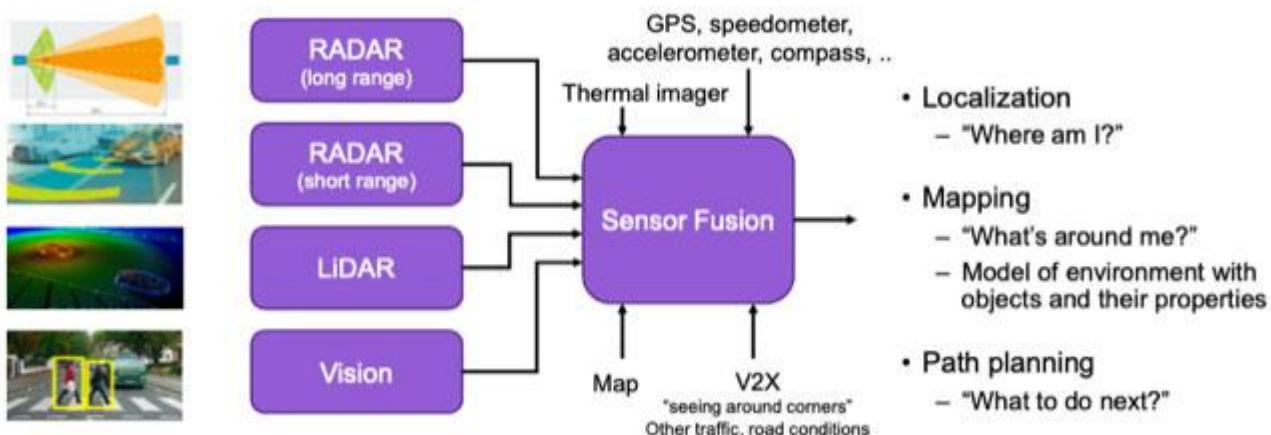
Sensor fusion in automotive designs integrates multiple sensors into a single chip, routing data intelligently. The goal is to combine information from cameras, radar, lidar, and other sensors for a comprehensive view inside and outside vehicles. Typically, this occurs in zonal controllers or central compute modules that collect sensor data and transmit it to a central unit. The location of sensor fusion and the sensors involved vary based on vehicle architecture and manufacturer approach.
