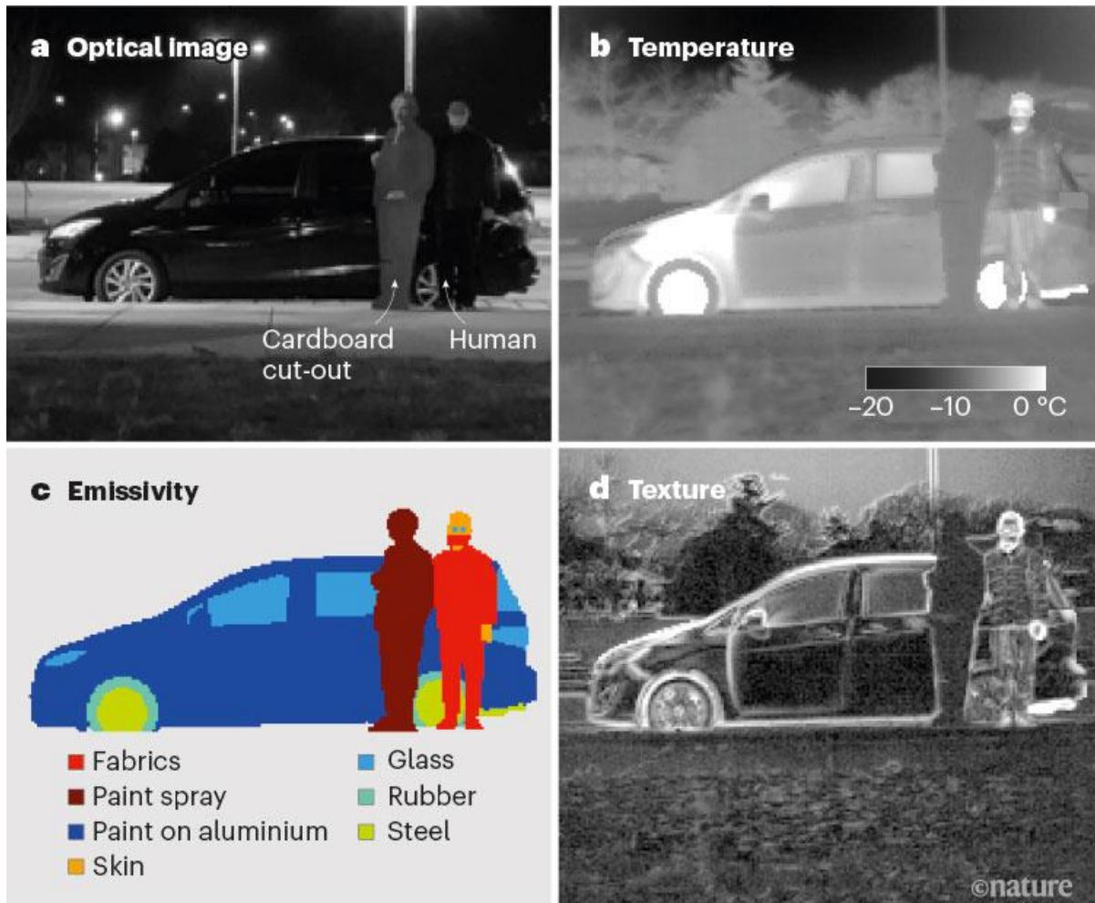
Heat-assisted detection and ranging (HADAR), a patent-pending thermal imaging technology from Purdue University, combines infrared (IR) imaging, machine learning, and thermal physics to visualize target objects in the dark as if it were broad daylight. According to its developers, the technology could have an impact on par with lidar, sonar, and radar, by enabling fully passive, physics-aware machine perception.
