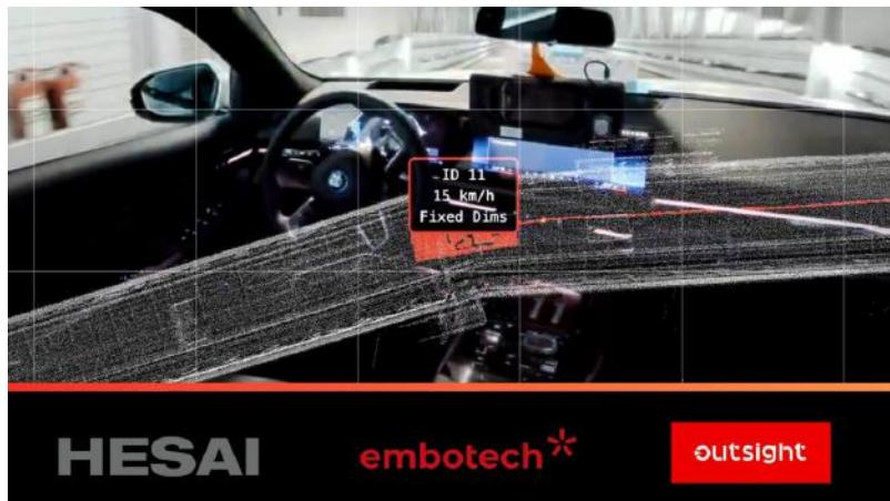
Lidar enables BMW's latest 5- and 7-Series models and their 0MINI Countryman to navigate autonomously to their finishing areas—showcasing the remarkable potential of this technology and spatial intelligence in modern manufacturing. As part of a commitment to automation, BMW began testing automated in-plant driving (AFW) at their Dingolfing plant, the largest in Europe. Using Outsight's RAD solution and feedback from advanced lidar
