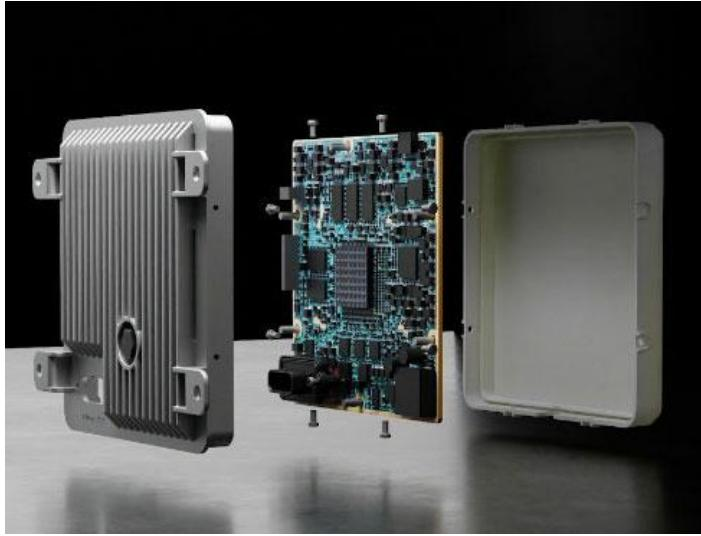
The Altos V2 shown here is the world's first mass-produced 4-chip cascaded imaging radar based on TI's TDA4. It boasts:
