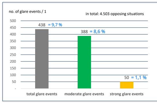
Split in 3 categories:Glare caused by:1. Asymmetry2. cut-off mis-aim3. Road topography
