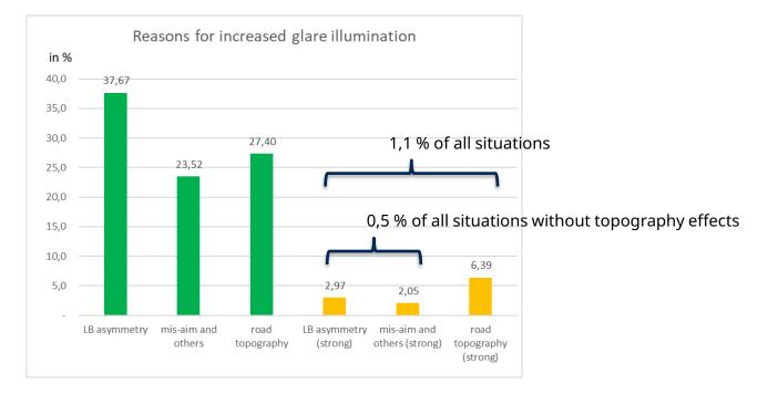
\* mis-aim and others: car inclination caused by load, mis-adjustment, high beam on, .....
