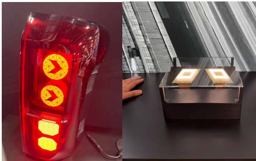
OLED rear lamp sample for e.g. trucks and a white OLED panel were shown.
