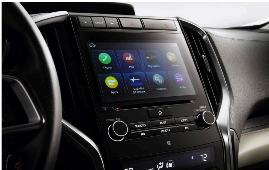
IMD COVER LENS AND IML MECHANICAL BUTTONS IN CENTER STACK (SUBARU IMAGE)
