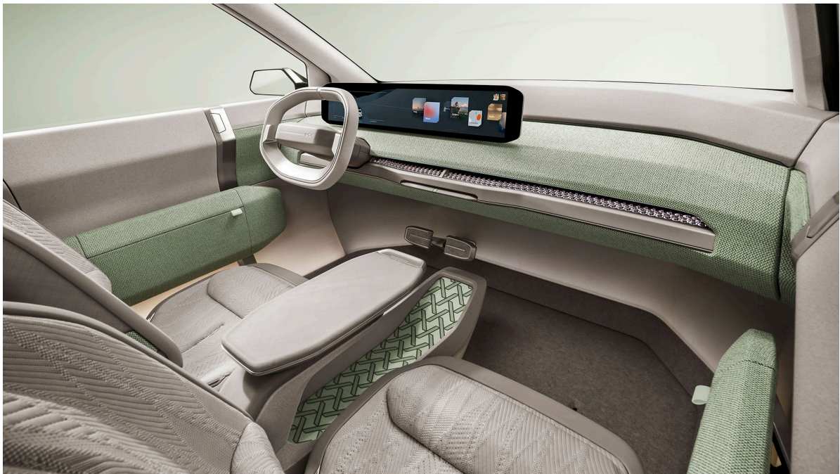
Kia wove fabric stripes by hand and applied them to create a 3D knit finish effect to the concept car's seat covers.
