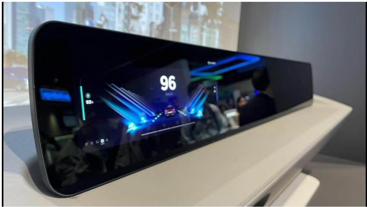
Curved cockpit design solutions with customizations and smart display and integrated sensing capabilities and seamless bonding are some of the other developments in pillar to pillar displays. The separation between screens seen here can be customized in such a way that when you are in the driver or passenger seat these boarders are not visible.
