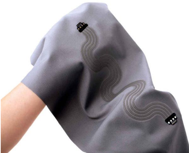
LOOMIA ELECTRONIC LAYER 4-WIRE BUS LAMINATED ONTO KNIT FABRIC (LOOMIA IMAGE)
