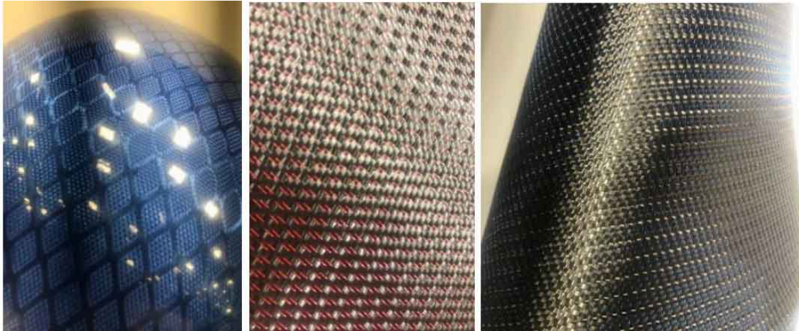
above and below: multi axial, and multi material fabrics showcasing Kevlar, carbon, glass, wool, copper, stainless steel, aluminum and optic fibers.
