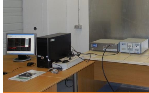
Test receiver for conducted and radiated emissions measurement
