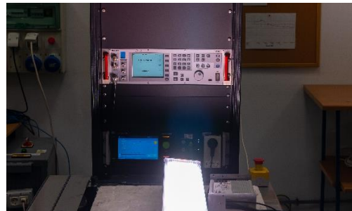
Multigenerator EM Test: surge burst, power fail, magnetic field.
