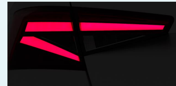
Rear Lamps Optic design full LED, realistic lit appearance, renderings and colorimetry analysis
