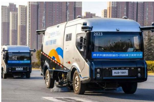
WeRide has deployed self-driving sanitation vehicles in Zhengzhou, Henan Province. The robosweepers feature  $L^4$  autonomous driving technology, operating at speeds of 5-10 km/h during sanitation work. Currently, the Zhengzhou Economic Development Zone autonomous sanitation project covers 16 complex urban roads, totaling 21.8 kilometers.
