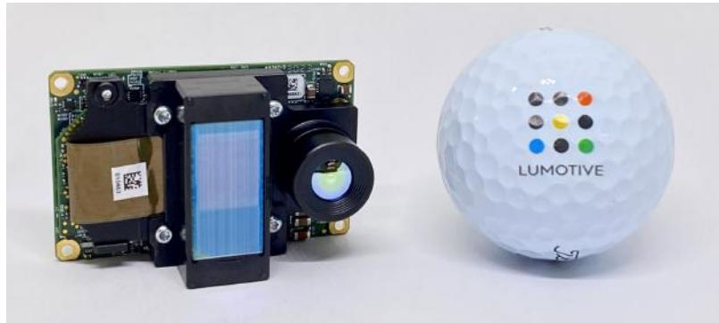
Lumotive won a CES Innovation Award for their LM10 LCM Module, which they call the world's first commercialised optical beam steering semiconductor. They say it offers true solid-state, zero-inertia beam steering, an ultrawide view field of up to 180° (with expansion optics), an 11 × 9 mm active aperture area to fit easily in a variety of system designs, and compatibility with all laser types, including VCSEL and EEL.
