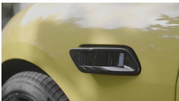
Speaking of the Lotus Emeya, it has two state-of-the-art RoboSense M Platform side lidar sensors. Lotus also put M Platform sensors on the Eletre, the company's first electric SUV, unveiled in March 2022. The sensor has a wide,  $120^\circ \times 25^\circ$  FoV, and can detect roadway objects at up to 200 m with 1.5 megapoints per second.
