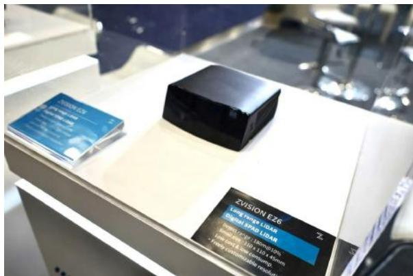
Chinese lidar provider Zvizon showed off their latest SPAD lidar, the EZ6. It's targeted for long-range ADAS applications. The maker says its 'novel architectural design' (which seems a bit bulky compared to the Lumotive M30 we just finished talking about....!) attains high chip-level integration for lower cost, (about USD \$280). With 192 channels, the EZ6 achieves point cloud characteristics with imagelike quality and improves the identification of low-lying obstacles.
