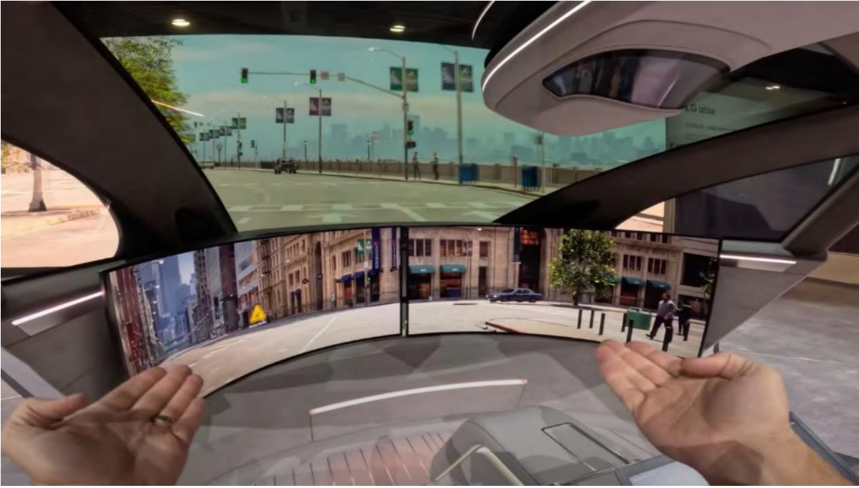
The αble recognizes hand gestures to reveal a second OLED screen up front
