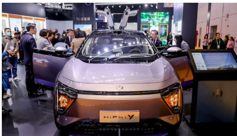
THE HIPHI Y HAS ADVANCED COVESTRO POLYCARBONATES, NOTABLY IN THE HEADLAMP AND LIDAR LENSES. (COVESTRO IMAGE)
