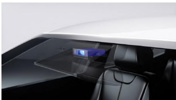
Hesai lidar will equip FAW's their next-generation EV under the Hongqi brand. It marks the 13th automaker to choose Hesai lidar, and the first series production design-in for their ultra-thin long-range ET25 lidar. The program is expected to begin mass production and delivery by H1-2025.
