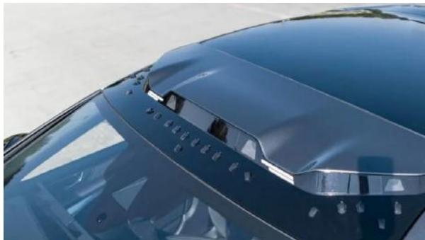
Hesai has partnered with Webasto for roof-mounted lidar sensor integration. Hesai will provide automotive lidar for Webasto's roof-mounted sensor modules designed for ADAS-enabled mass production vehicles. The AT128 lidar seamlessly integrates into the roof sensor module, while the slim ET25 lidar can be discreetly placed behind the windshield, offering a unique interior installation that complements vehicle design, maintains aerodynamics, and remains resistant to dirt and debris.
