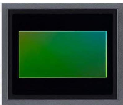
Sony Semiconductor Solutions will release their IMX735, a new CMOS image sensor for automotive cameras with what they're calling the industry's highest pixel count—17.42 megapixels—enabling high-definition capture of far-off objects. Most CMOS sensors read signal output from pixels one vertical line at a time, but the IMX735 outputs signals horizontally, one row at a time. This lets automotive cameras more easily synchronize with mechanical scanning lidar.
