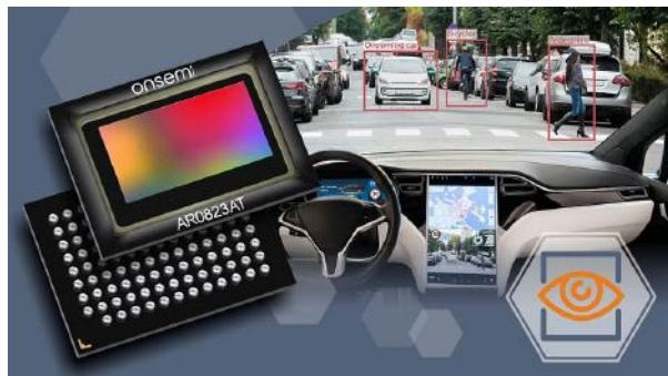
**Onsemi:** This major silicon supplier demonstrated their Hyperlux automotive image sensor. With a  $2.1 \mu\text{m}$  pixel size, 150-dB ultra high dynamic range and LED flicker mitigation across the full automotive temperature range, the Hyperlux provides high performance and speed and advanced features for ADAS. This technology enables  $L^{2+}$  driving automation.
