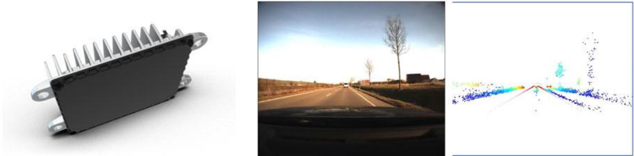
Road scene video and corresponding Imaging Radar 3D point cloud
