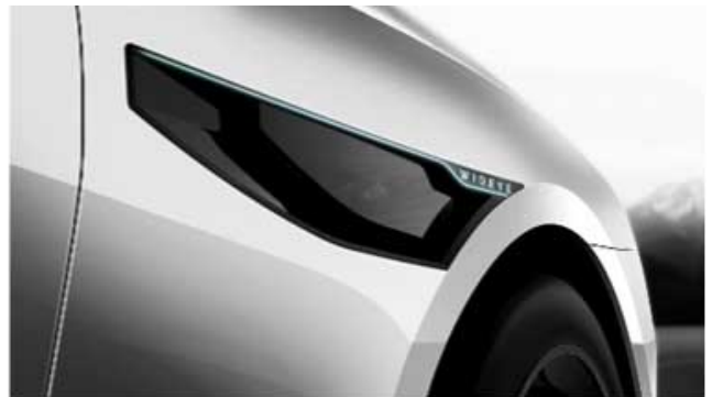
Side lidar integration: a sensor mounted seamlessly and aesthetically on the fender
