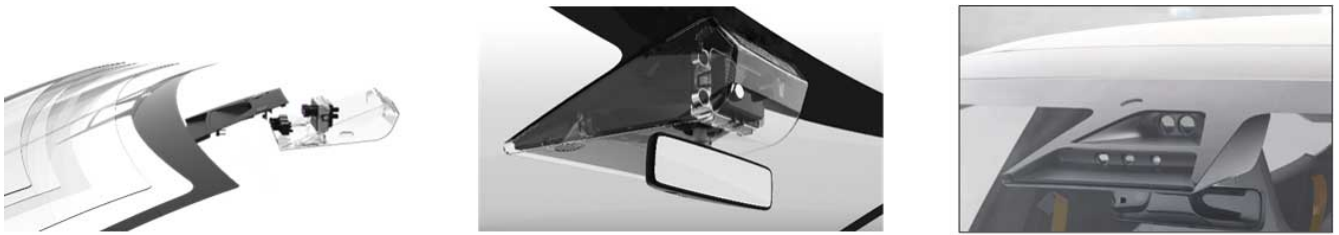
Integration of a lidar and cameras module behind the windshield
