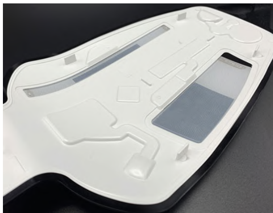
VERSO OF IMSE LIGHTCHANNELS DEMONSTRATOR AFTER SECOND SHOT OF INJECTION MOLDING (TACTOTEK IMAGE)
