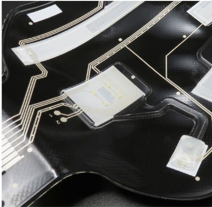
INJECTION-MOLDED CHANNELS CONTROLLING LIGHT (TACTOTEK IMAGE)
