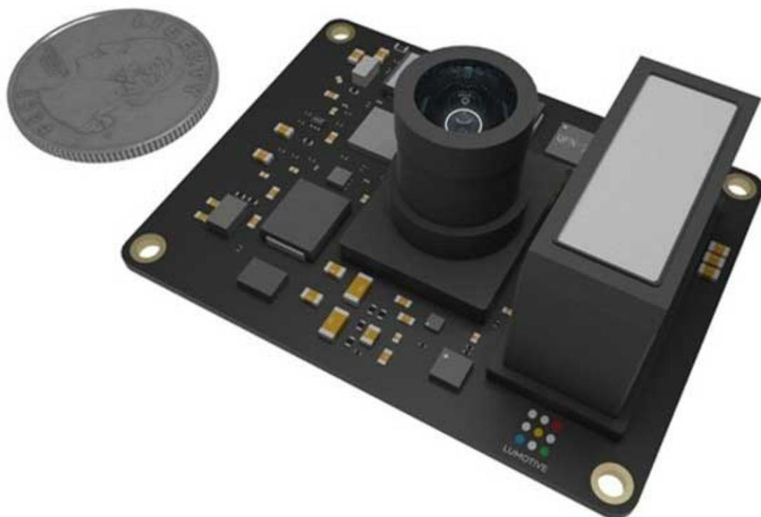
Lumotive and Lumentum Holdings have announced availability of the M30 Reference Design, a complete sensor implementation of their software-defined lidar solution. The design integrates Lumotive's Light Control Metasurface (LCM) beam steering chips and Lumentum's M52-100 multi-junction VCSEL array. Lumotive demonstrated the LCM beam steering technology at SPIE Photonics West 2023 in San Francisco.
