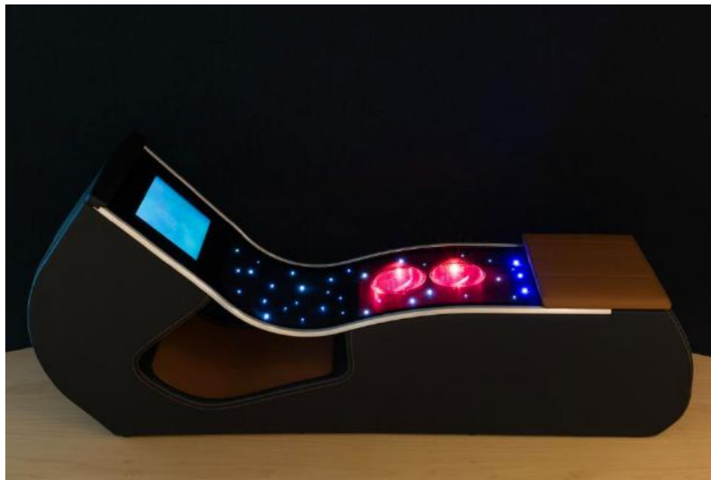
CONSOLE PROTOTYPE: LEDS IN POLYCARBONATE WITH HAPTIC TOUCH TO CONTROL THE STAR FIELD. (ROB MILLER IMAGE/DVN)
