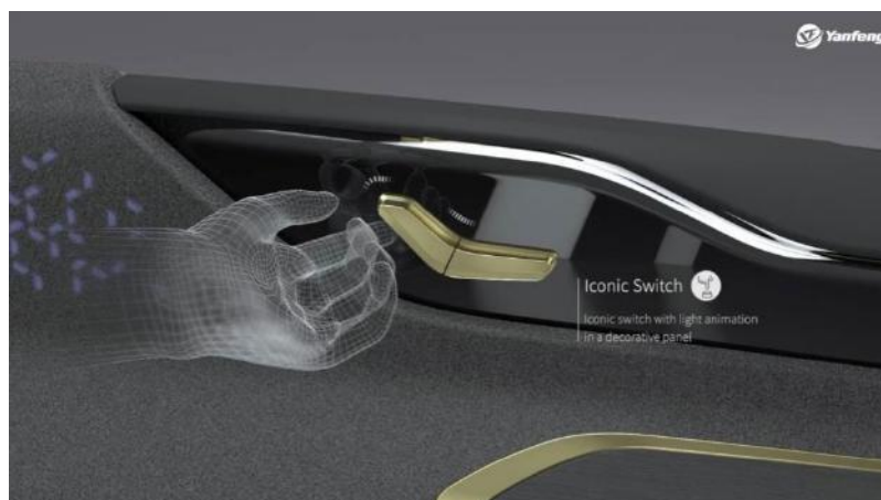
HAPTIC TOUCH WITH VISUAL FEEDBACK ON PLASTIC DOOR PANELS (YANFENG IMAGE)
