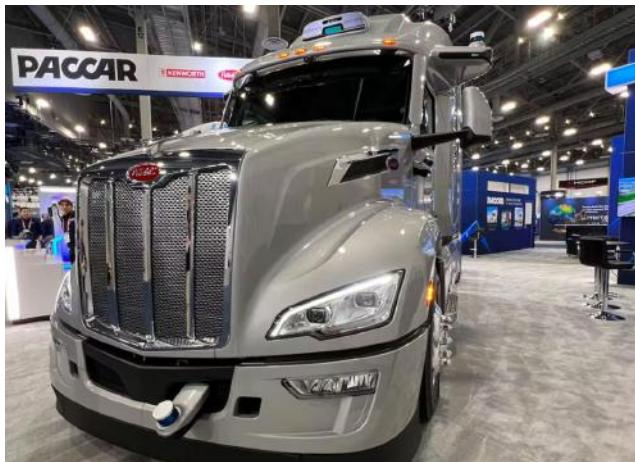
Paccar has been showing off their Peterbilt 579 equipped with lidar and cameras. The vehicle is L4-capable and is currently running pilots with Aurora in West Texas.
