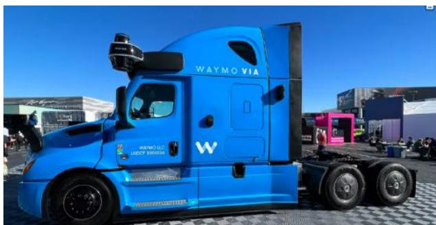
The special Cascadia is equipped with a fifth-generation Waymo Driver. About 50 of these early-build pilot trucks are operating in Texas and Arizona with Uber Freight; J.B. Hunt, and others. And a revised 'beta' build of this model is said to be coming soon.
