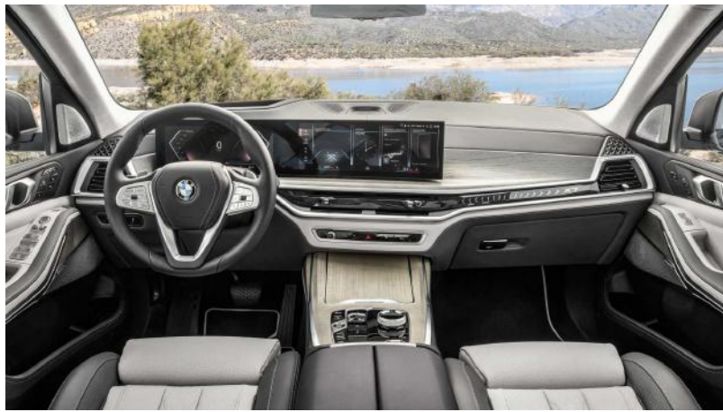
BMW X7 COCKPIT CURVED DISPLAY: 12.3" INSTRUMENT CLUSTER WITH 14.9" MAIN SCREEN (BMW IMAGE)
