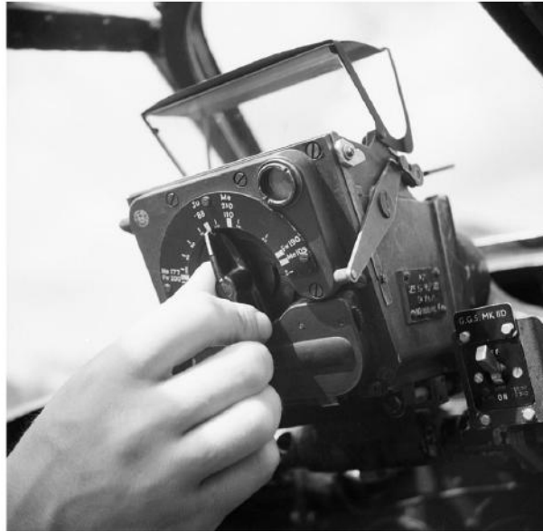
GYROSCOPIC GUNSIGHT IN SUPERMARINE SPITFIRE (WIKIPEDIA IMAGE)
