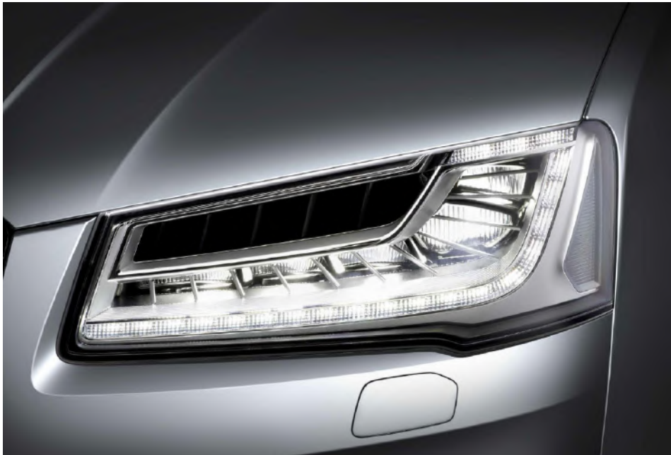
MATRIX LED HEADLAMPS WITH GLARE-FREE HIGH BEAM IN AN AUDI A8 (HELLA IMAGE)
