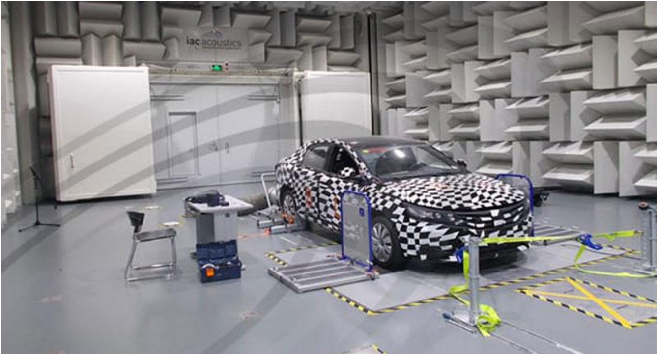
VSAC: VEHICLE SEMI-ANECHOIC CHAMBER (IAC ACOUSTICS IMAGE)
