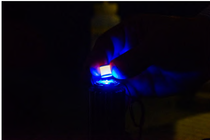
DOWN-CONVERTING PHOSPHOR CONVERTING BLUE LIGHT INTO A CUSTOM WHITE LIGHT (LUMENFLOW IMAGE)
