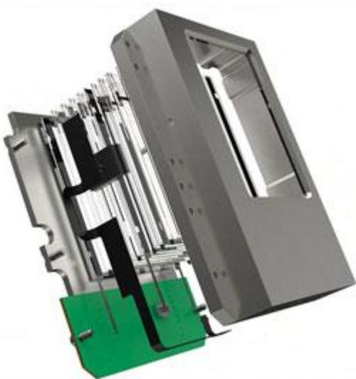
LeddarSteer is available to lidar makers and tier-1 suppliers for the design and production of long-range, high-resolution lidars in a complete solid-state form—with no moving parts to wear out or to be affected by shocks and vibrations present in an automotive environment.
