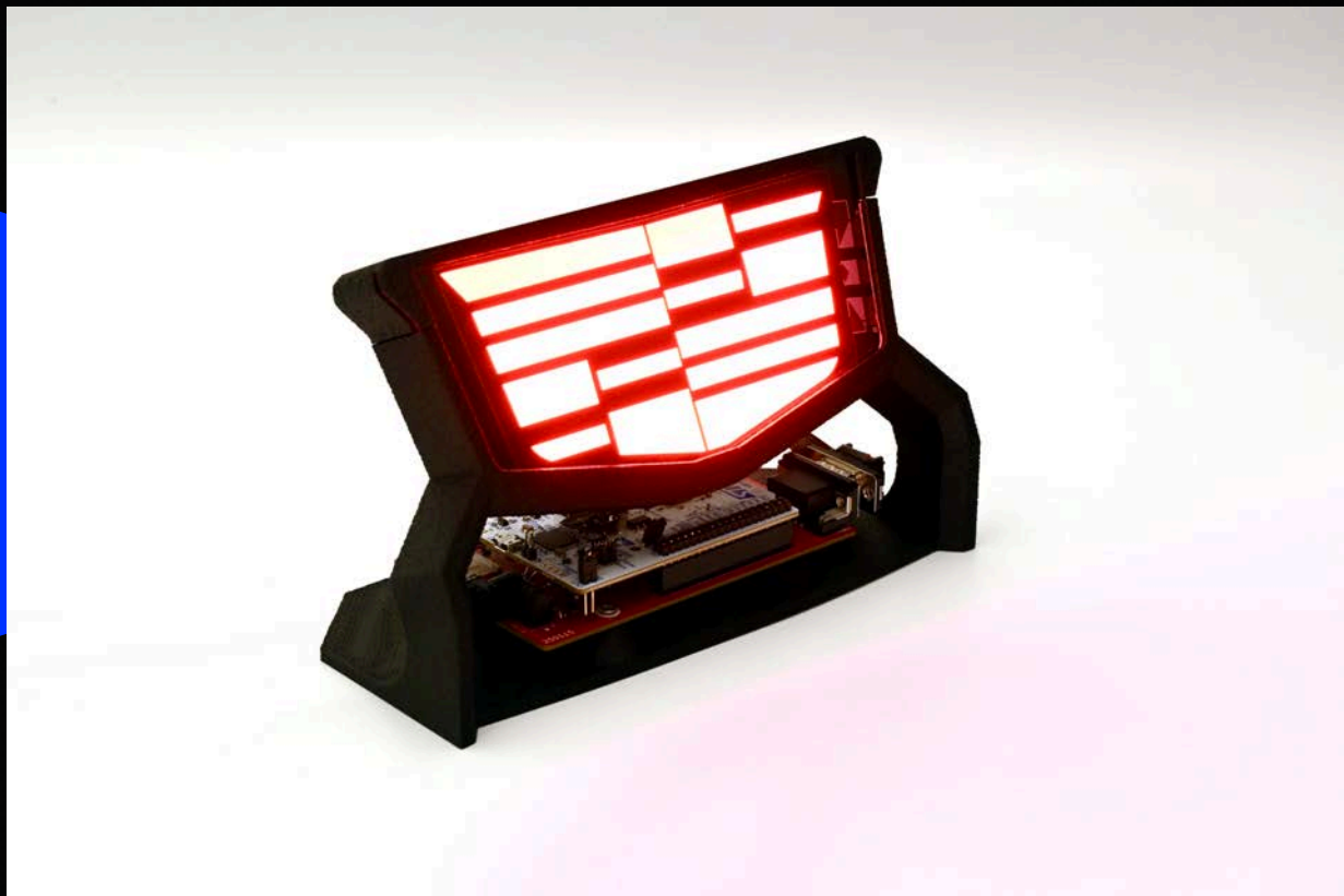
Prototype of red Cadillac badge using Atala Digital technology
