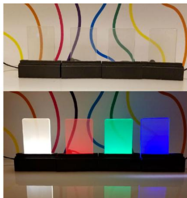
FOUR IDENTICAL 50 × 75 MM CHIPS OF MAKROLON Ai2215 EL WITH NO ILLUMINATION (TOP) AND WITH WHITE, RED, GREEN, AND BLUE LEDs ILLUMINATING THE BOTTOM EDGE (BOTTOM). RED, GREEN AND BLUE CAN BE BLENDED TO MAKE ANY COLORS.
