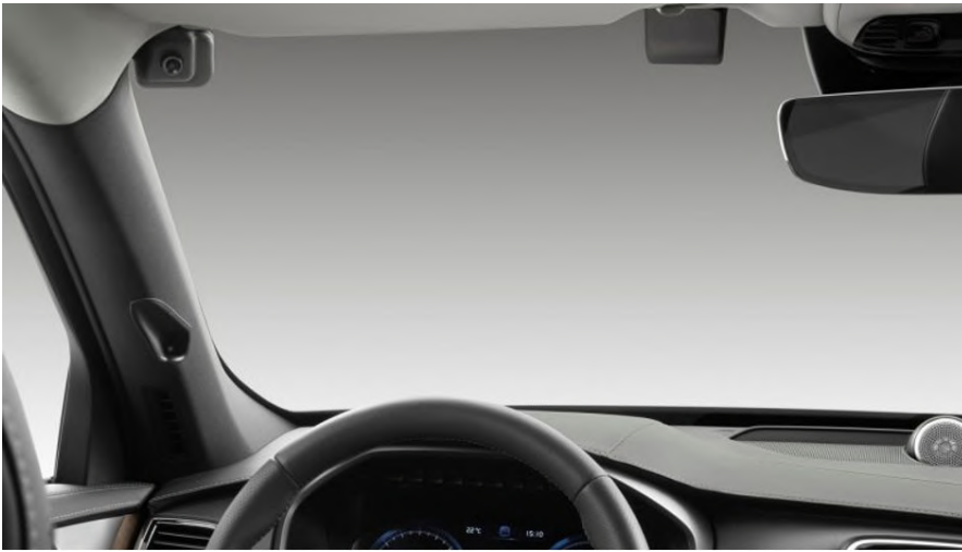
DMS CAMERA IN VOLVO RESEARCH VEHICLE, UPPER LEFT. SECOND CAMERA IS ON FAR RIGHT OF WINDSHIELD.
