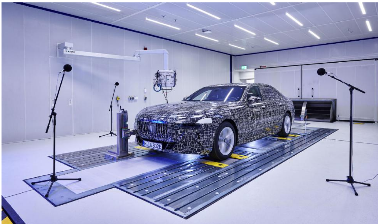
A CAMOUFLAGED NEW I7 IN DEVELOPMENT ON AN ACOUSTIC TEST BENCH (BMW IMAGE)
