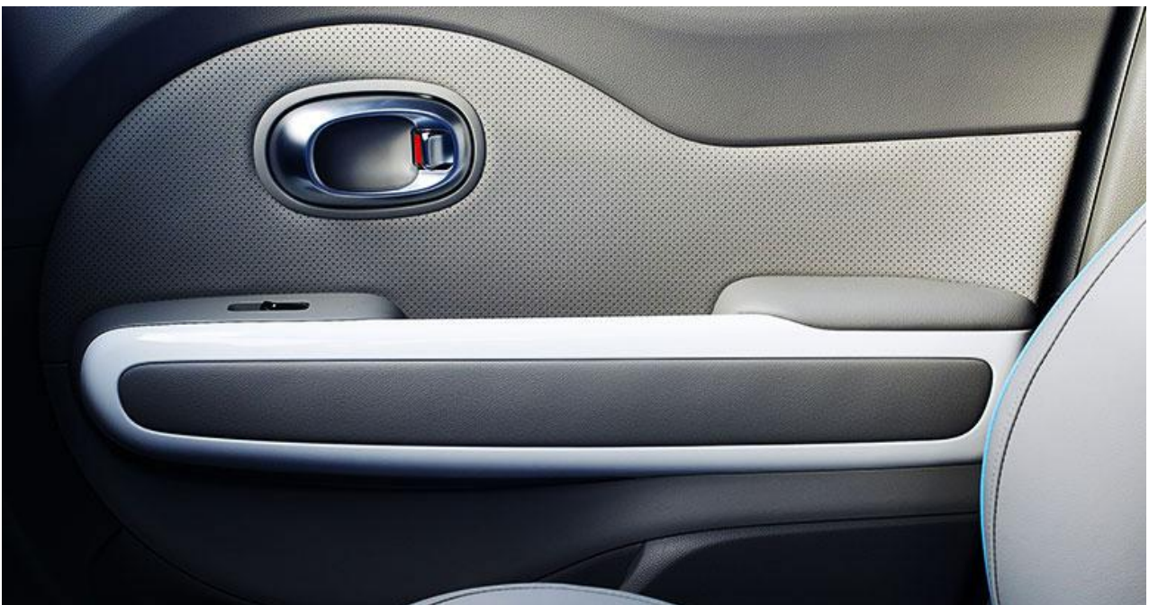
KIA SOUL EV DOOR TRIMS MADE OF SUGARCANE AND WOOD-EXTRACTED BIOPLASTIC. (KIA IMAGE)
