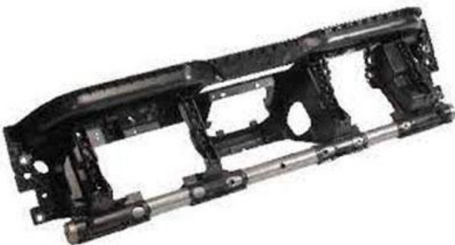
LIGHTWEIGHT HYBRID STEEL/GMT COMPOSITE IP CARRIER (FAURECIA IMAGE)
