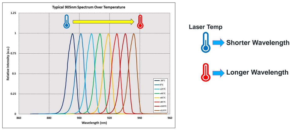
LiDAR sensor designs must consider this behavior in the optical path from Tx to Rx.
