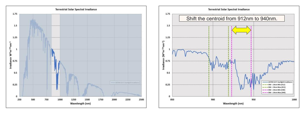
Reduced sun load impact can improve SNR for LiDAR sensors.
