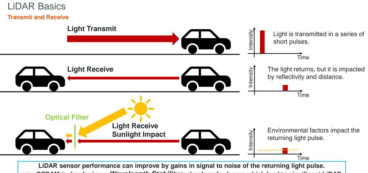
ams OSRAM is developing a *Wavelength Stability* technology for lasers which lead to significant LiDAR performance improvements.
