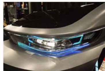
Headlamp module with LiDAR
