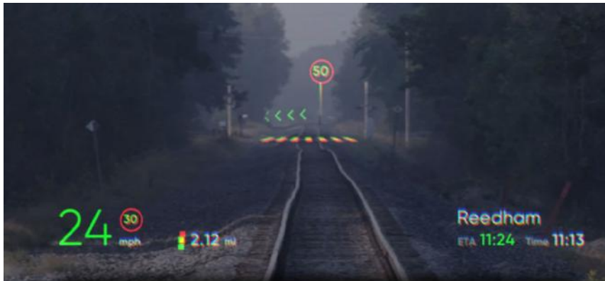
HOLOGRAPHIC AR-HUD FOR VERSATILE TRANSPORT VEHICLES (WAYRAY IMAGE)
