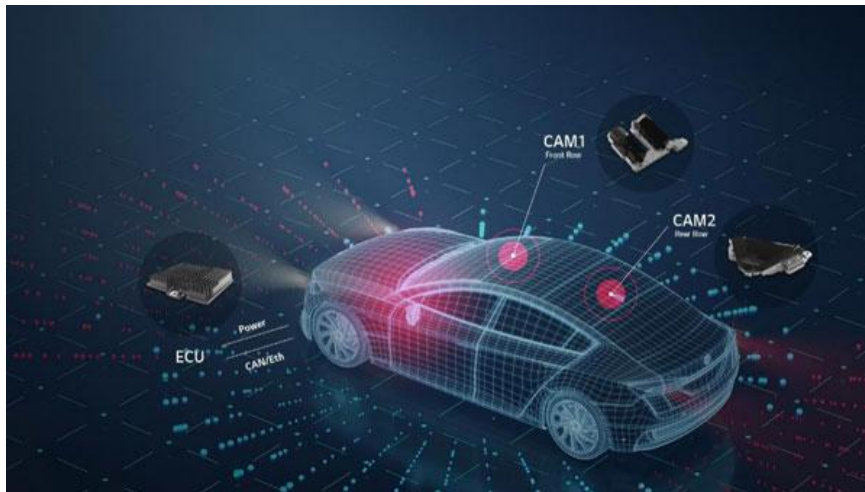
LG CABIN CAMERA ARCHITECTURE (LG IMAGE)
