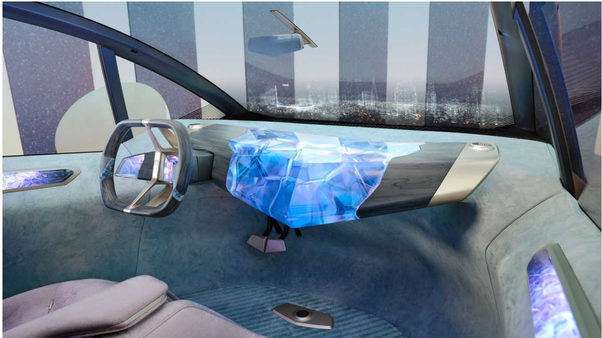
3D-PRINTED PANELS WITH GLASS & WOOD EXTEND REARWARD FROM THE IP (BMW IMAGE)
