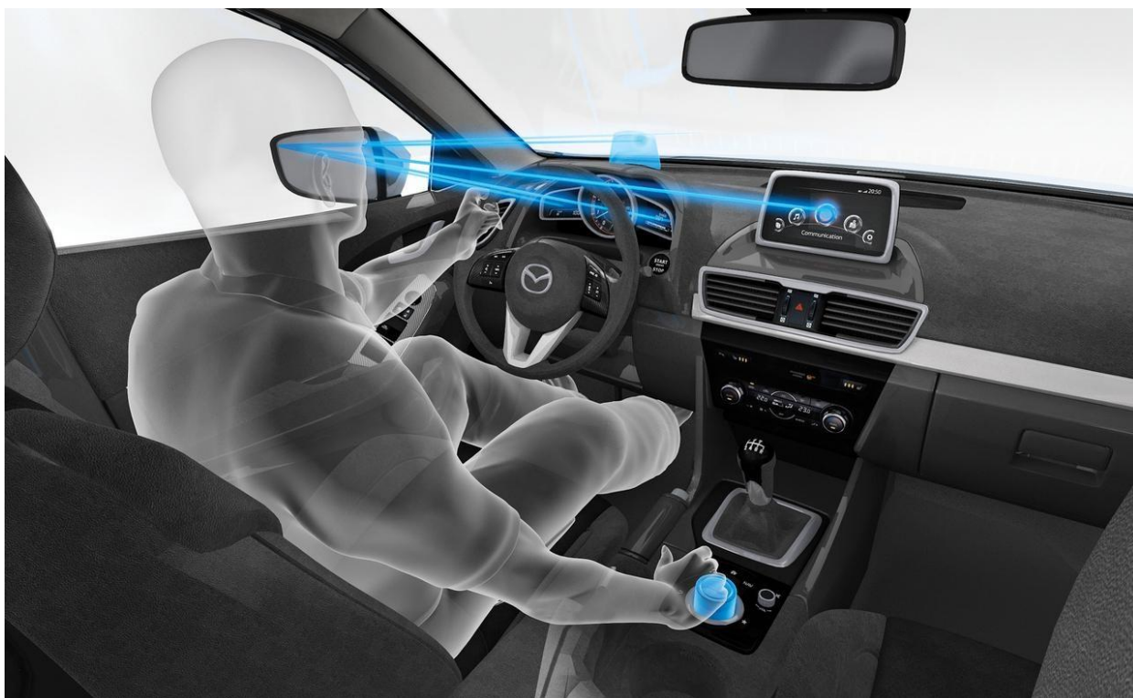
EYE-BASED DRIVER MONITORING SYSTEM (HARMAN)
