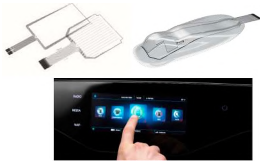
CAPACITIVE TOUCH SENSORS WITH TRANSPARENT AND CONDUCTIVE FILMS (IMAGE: POLYIC)
