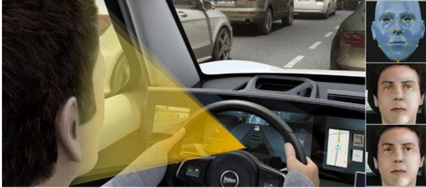
DRIVER MONITORING: A CAMERA TO MONITOR DRIVER ALERTNESS (VALEO)
