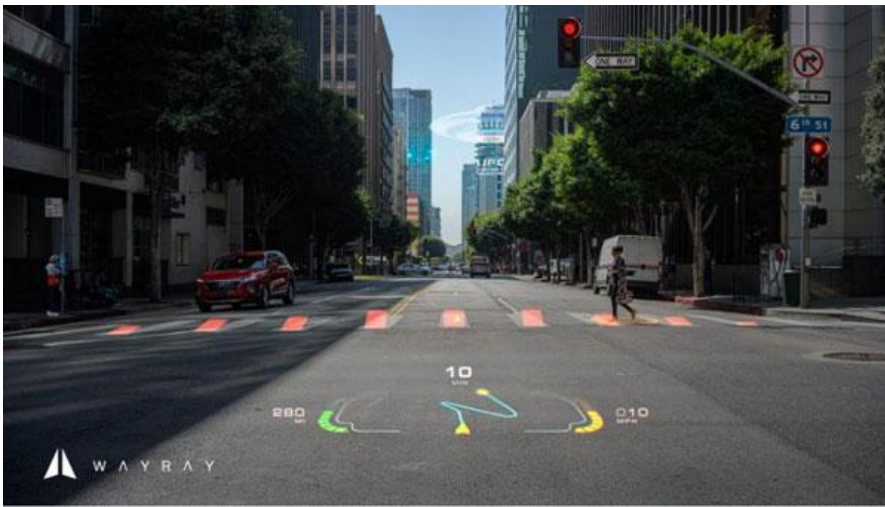
WAYRAY FULL-COLOR HOLOGRAPHIC AR DISPLAY (IMAGE: WAYRAY)
