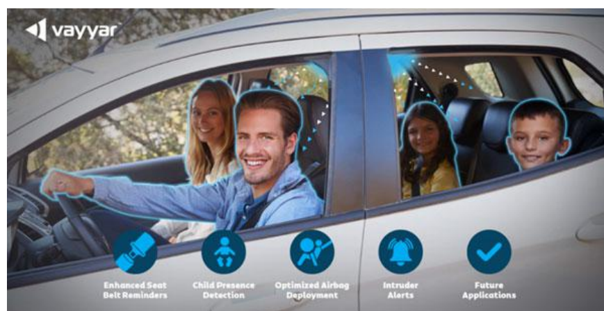
A single Vayyar sensor monitors two complete seating rows and the presence of five occupants, replacing several in-car sensors.
